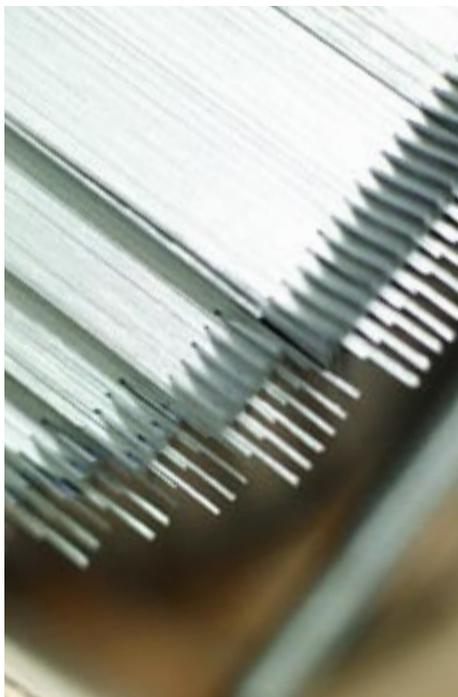
Whether in design, manufacturing methods or materials – the cores of Siemens transformers represent the latest state of technology. The silicon-alloyed electric sheet steel used is grain-oriented, cold-rolled and insulated on both sides, guaranteeing low losses and noise – and these values are even improved by laser treatment.
