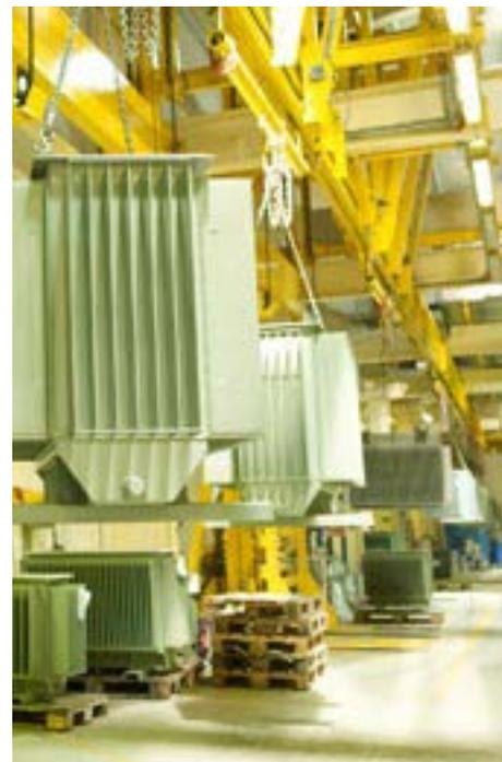
Whether during transport or operation – the tank must be absolutely tight under mechanical stress. Preconditions to achieve this are constructional experience, the most modern calculation methods and high-quality welding work.
